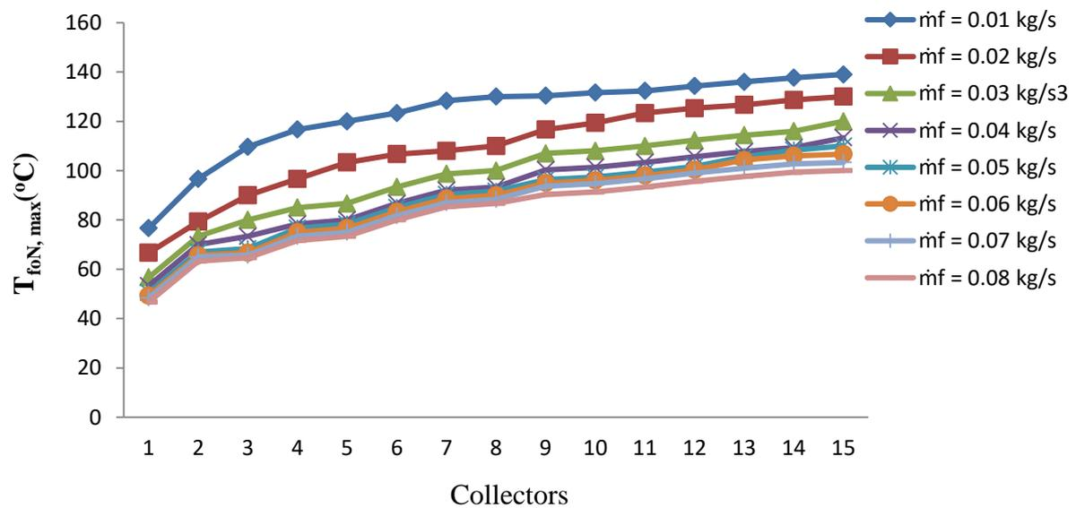
Fig. 5 for Dual inclined water temperature collector ( $T_{woN,max}$ ) in the month of June
