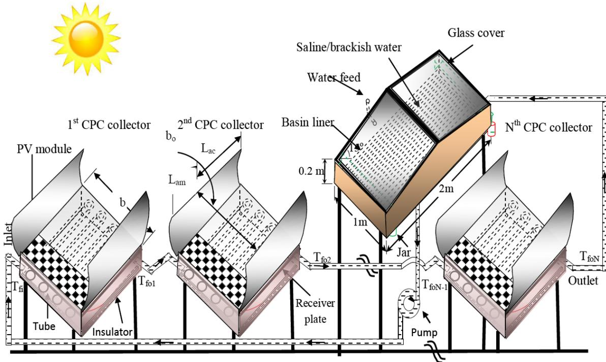
**Fig. 2** Dual inclined PVT-CPC active solar filtration system
