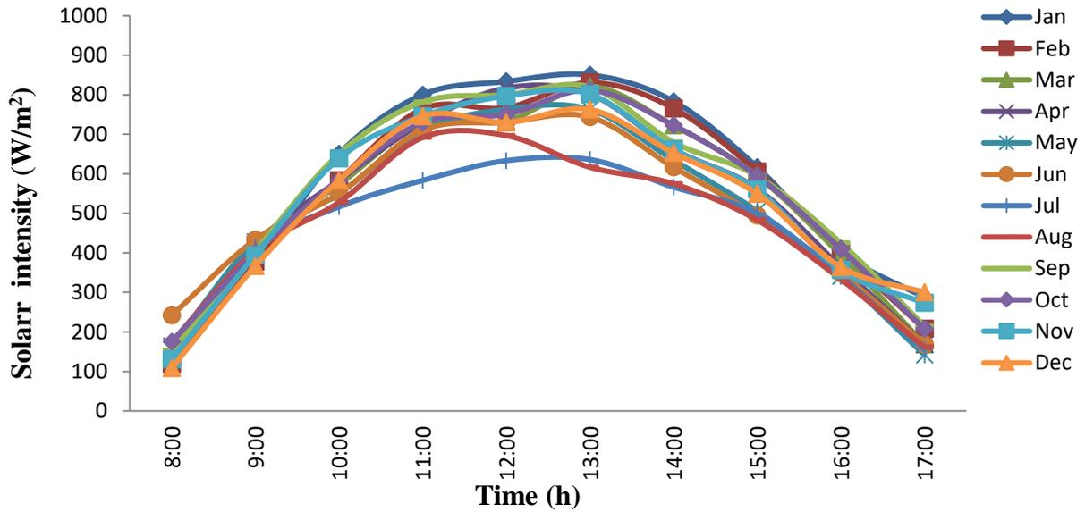
Fig 3 per hour variation of the beam radiation ( $I_b$ ) month-wise
