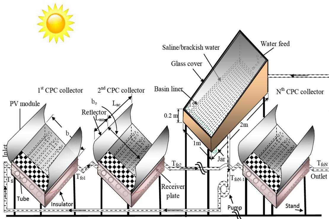
Fig. 1 Solo inclined PVT-CPC active solar filtration system
