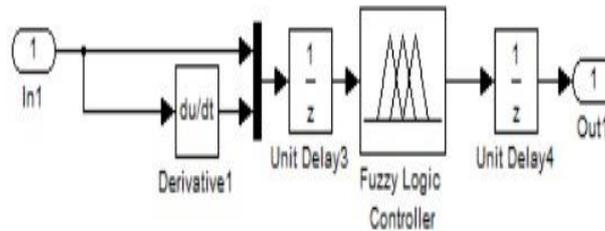
**Fig. 7.** Fuzzy Logic Controller Simulink Model.
