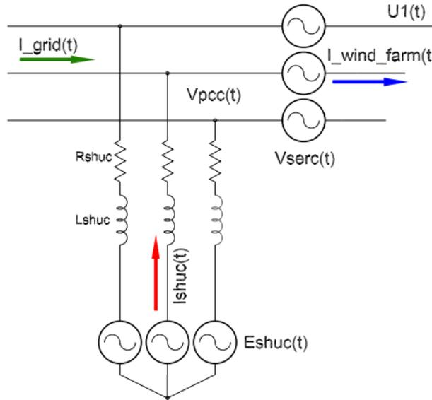
**Fig. 4.** Power stage compensator model-AC Side.
