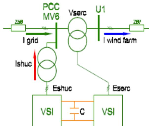
Fig. 2. Block diagram of UPQC.
