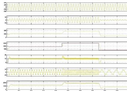
**Fig. 2.** Proposed FLC Controller Simulation Outcomes. (a) Sending Source Voltage, Vss vs Time, (b) Sending Source Current, Iss Vs Time, (c) dc Voltage Vs Time, (d) Speed, Speed reference Vs Time, (e)Torque, limiter Vs Time (f) Average Current, Vs Time, (g)Imean Vs Time.
