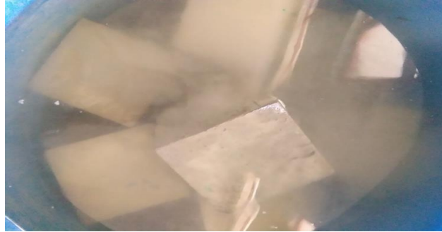
Casted specimen in curing tank
