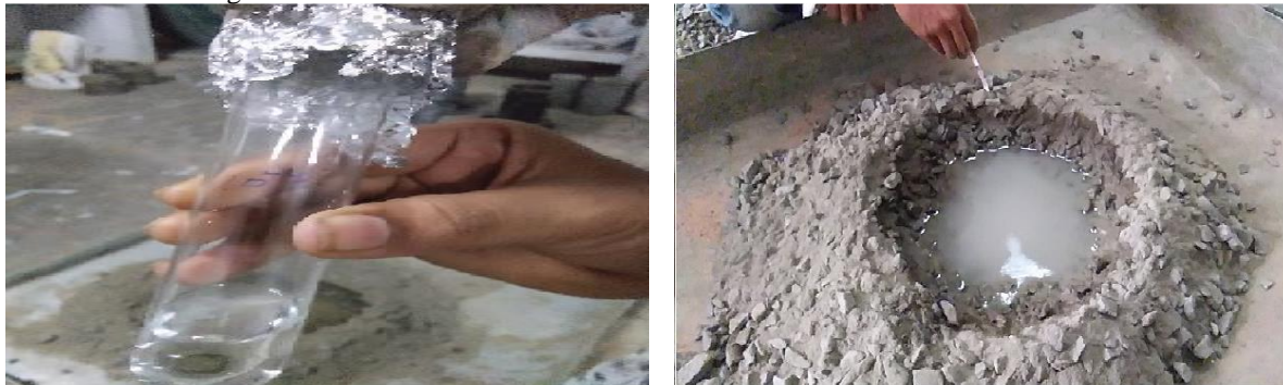
Bacteria with concentration before mix View of addition of Bacteria in concrete
