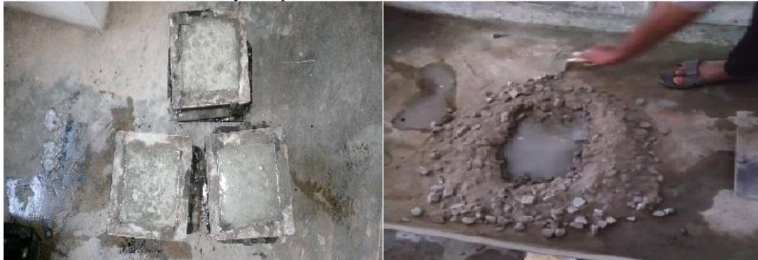
Mixing, Placing and Compaction done for the concrete cubes
