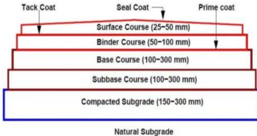
Typical Cross-section of a flexible pavement
