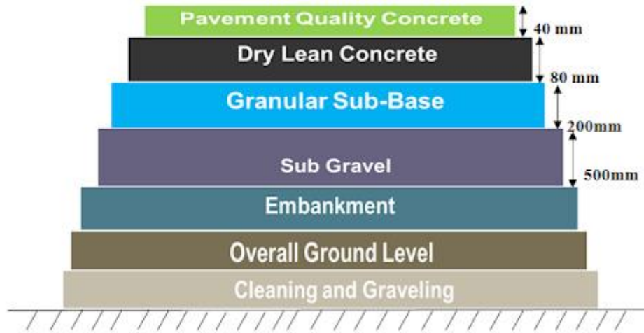
Layers in Rigid pavement
