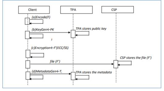
The Metadata For Each File Is Computed By The Client To Verify The Integrity Of Cloud-Stored Data.
