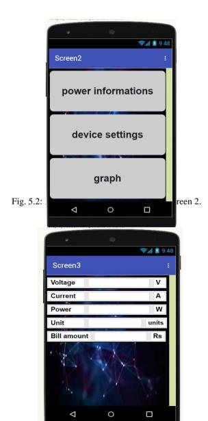
Figure. 5.3: MIT App Inventor Blocks Editor Screen 3 – User can monitor the voltage, current, power consumption unit , and also the bill amount in the text box provided.
