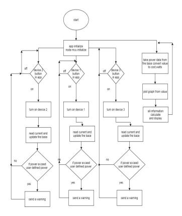
Figure 4.2 Flow chart of IOT based power depiction system .
