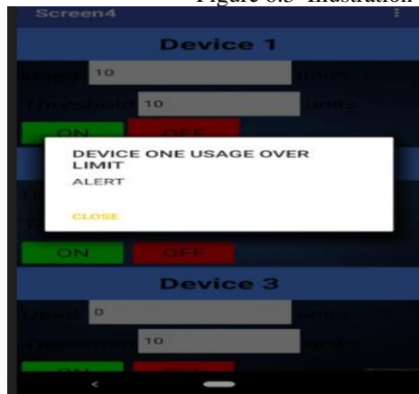
Figure 6.4 Image of alert message popup when threshold exceeds.
