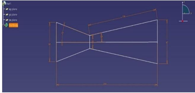
**Figure 1:** The dimensions marked at the CD nozzle as per in the Table 1 (Case 1)
