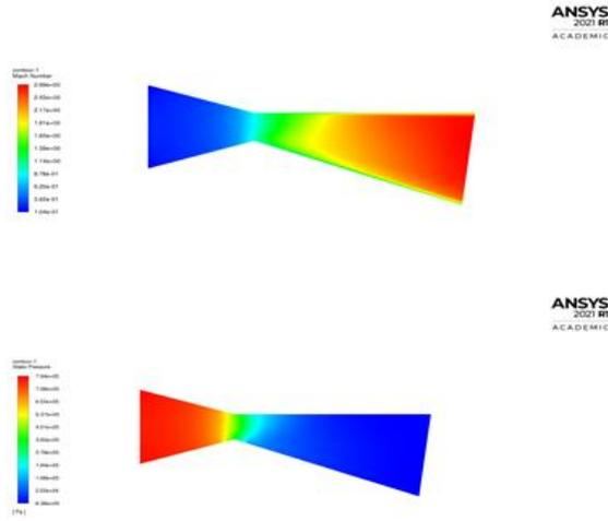
**Figure 9:** The mach (top) and pressure (bottom) are contours of Case 3 (10°) CD nozzle.
