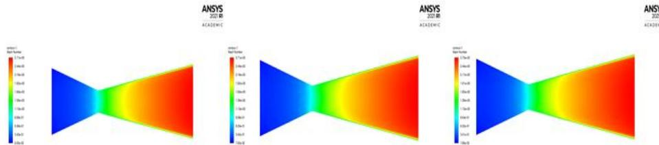
**Figure 17:** The mach contours of the meshing with number of divisions of 350 (left), 400 (middle), 450 (right) respectively
