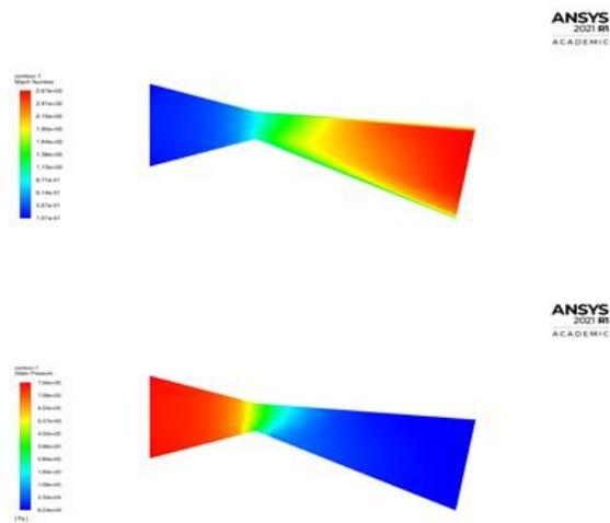
**Figure 10:** The mach (top) and pressure (bottom) are contours of Case 4 (15°) CD nozzle.
