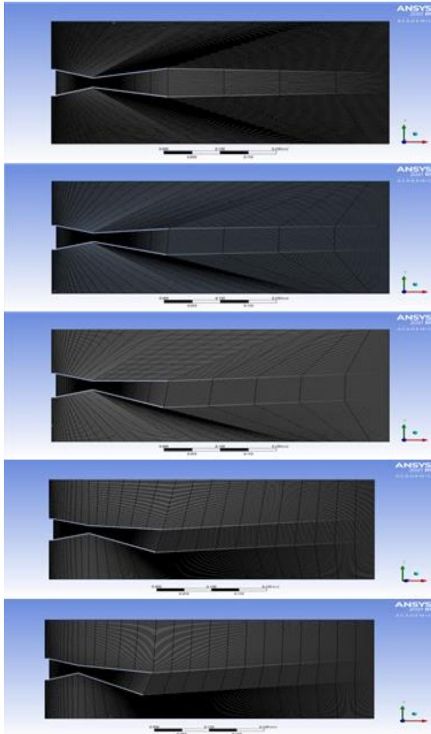
**Figure 6:** Meshed nozzle with domain of the Case 1, 2, 3, 4 & 5 (top to bottom)
