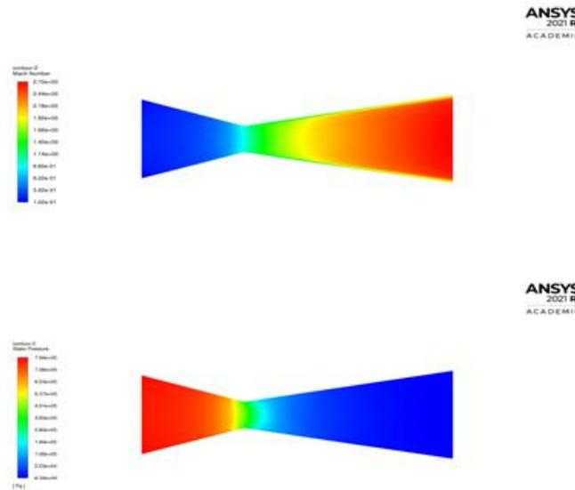
**Figure 7:** The mach (top) and pressure (bottom)are contours of Case 1 (0°) CD nozzle.
