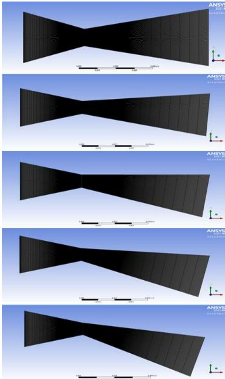
**Figure 5:** Meshed nozzle of the Case 1, 2, 3, 4 & 5 (top to bottom)
