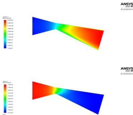
**Figure 11:** The mach (top) and pressure (bottom) are contours of Case 5 (20°) CD nozzle.
