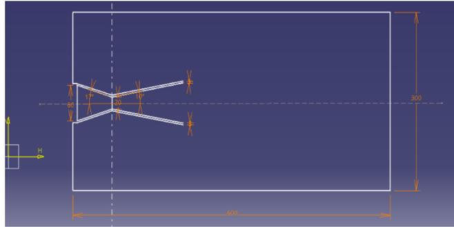
**Figure 3:** The dimensions marked at the CD nozzle with domain as per in the Table 1 (Case 1)
