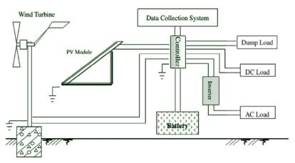
Fig. 1 Block Diagram of Solar Wind Hybrid System [5]
