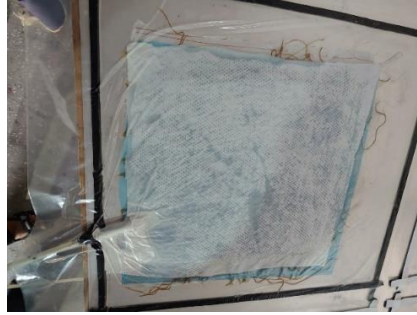
Figure 3.2 (Vacuum Infusion Method)
