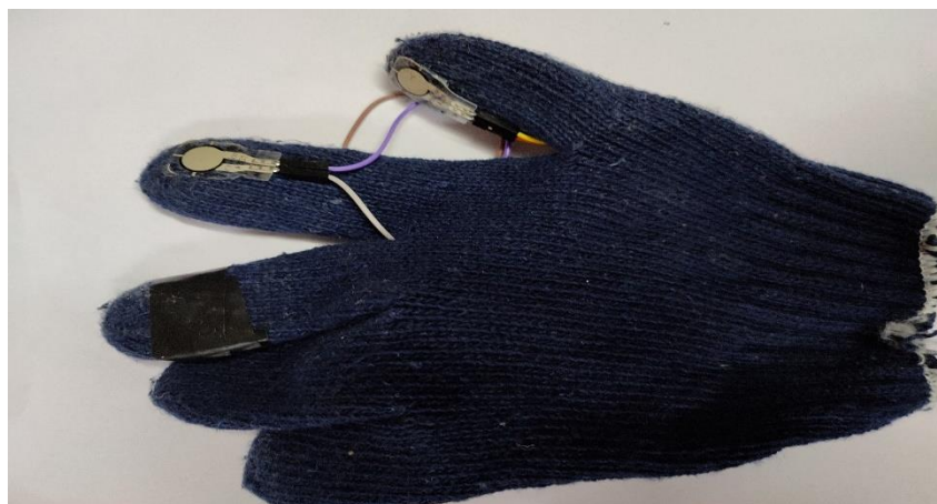
Figure 1. A301 Flexi force sensors on finger tips of index and thumb finger of a glove.
