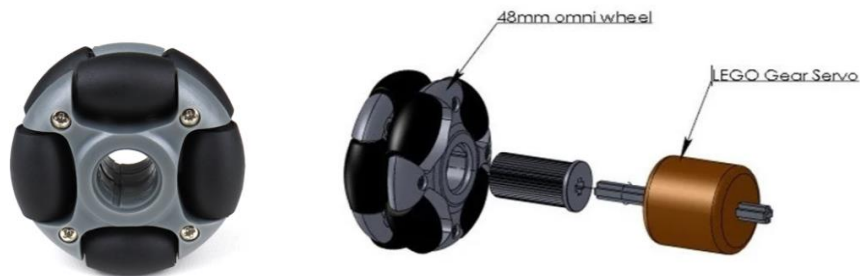
Fig. 12. (a) 48mm dia Omni wheels
