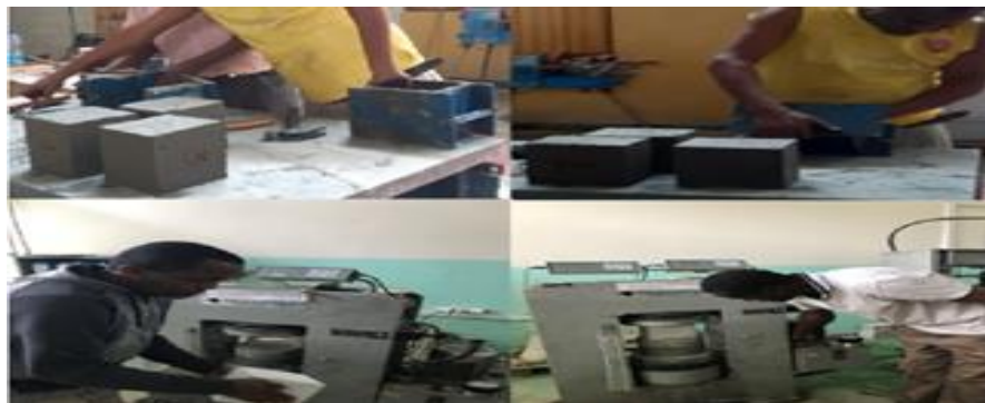
Figure 1.1 Testing compressive strength of cube samples
