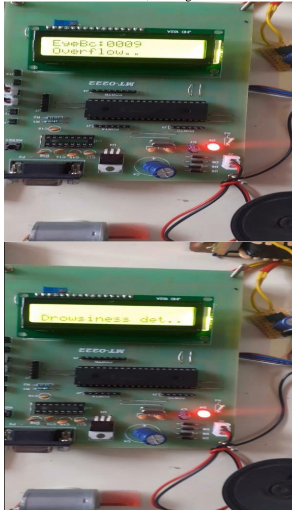
Fig. 9 If e/s greater than 5 e/s than the drowsiness detection will be given in the form of voice.
