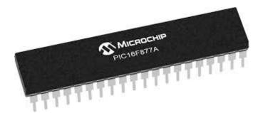
Fig.2 PIC Microcontroller
