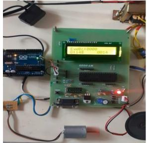
Fig. 7 Speed of the motor is reduce when the distance is less than the threshold value and alert in the form of voice will also be given
