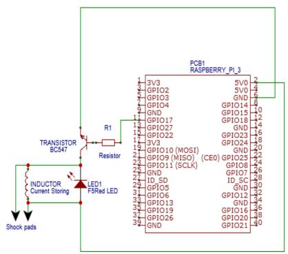
Figure 3: Circuit diagram
