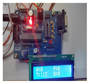
Fig 3f. ABNORMAL TEMPERATURE READING
