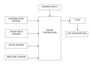
Fig 1 Transmitter Section
