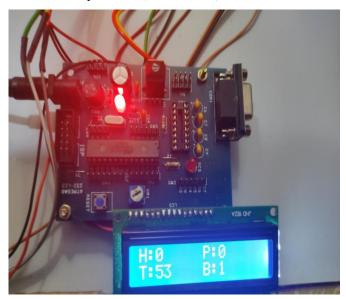
Fig 3c. EXHALATION READING IN LCD
