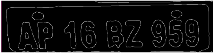
Fig. 8. Contour Detection with the Contours of various Imperfections
