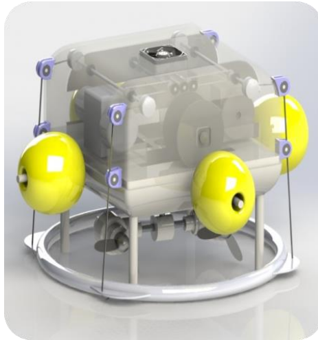
Fig: 1.3 Micro-Bubble Aerator
