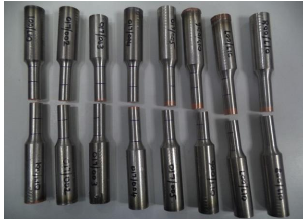
Fig. 4. Fractured samples after tensile test.
