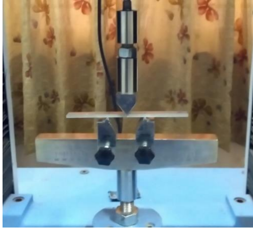
Fig. 6. Flexural test set-up
