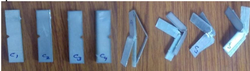
Fig. 13. Charpy Impact test specimen before and after impact.
