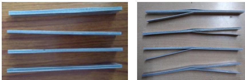
Fig. 9. Flexural test Specimen Before and after test.
