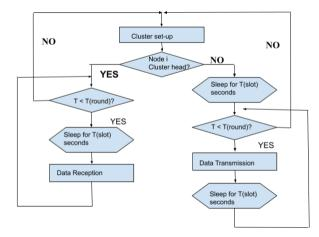
Fig. 2. Steady-state stage: LEACH Protocol
