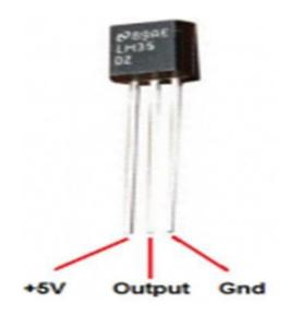
**Figure: Temperature sensor**
