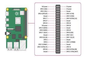
Figure: Pin description of Raspberry pi
