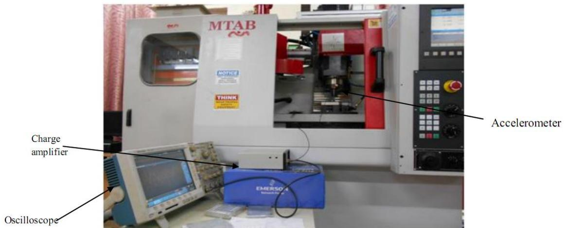
**Figure 6. Experimental set up for the cutting tests**
