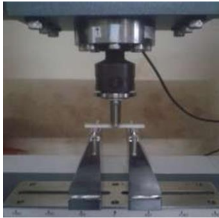
Fig.4. Bending Test setup
