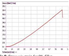
Fig.8; Stress v/s strain for 9% filler
