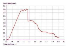
Fig.9 Stress v/s strain without filler
