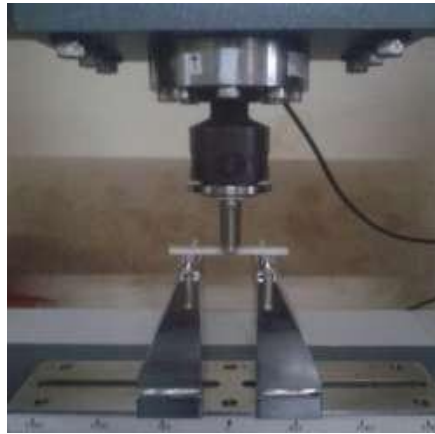
Fig.4. Bending Test setup
