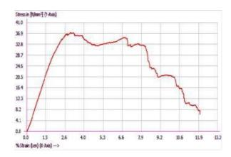
Fig.11 Stress v/s strain for 9% filler
