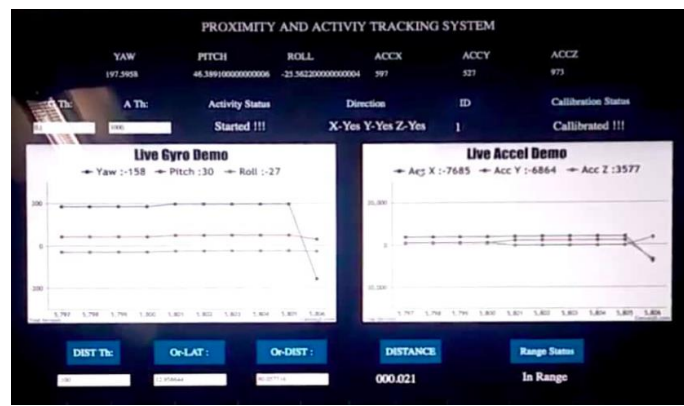
Fig. 8: Webpage plotting real-time data transmitted from the prototype.
