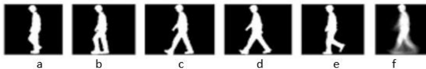
Fig.2. (a-e) Binary silhouette images in a gait sequence, (f) Corresponding GEI Image
