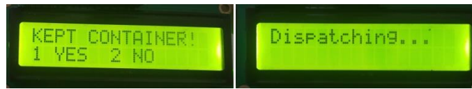
Fig 10: Requesting to select container presence at the dispatcher
