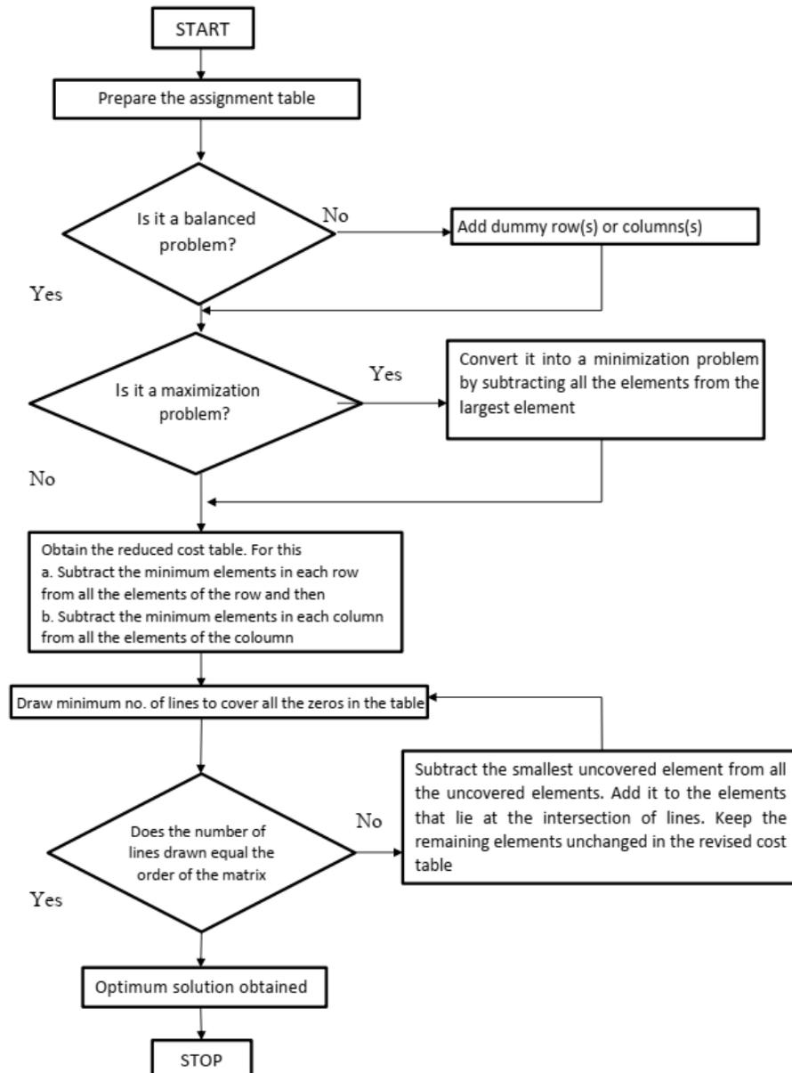
**Figure 1: Flowchart for Hungarian assignment method for course Timetabling.**
