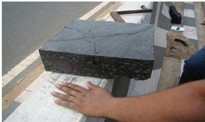
Fig.6 Cracking pattern identified during coring
