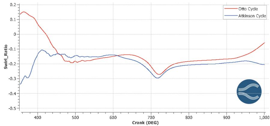
**Figure 4.11** Swirl ratio comparison between Otto cycle and Atkinson cycle.
