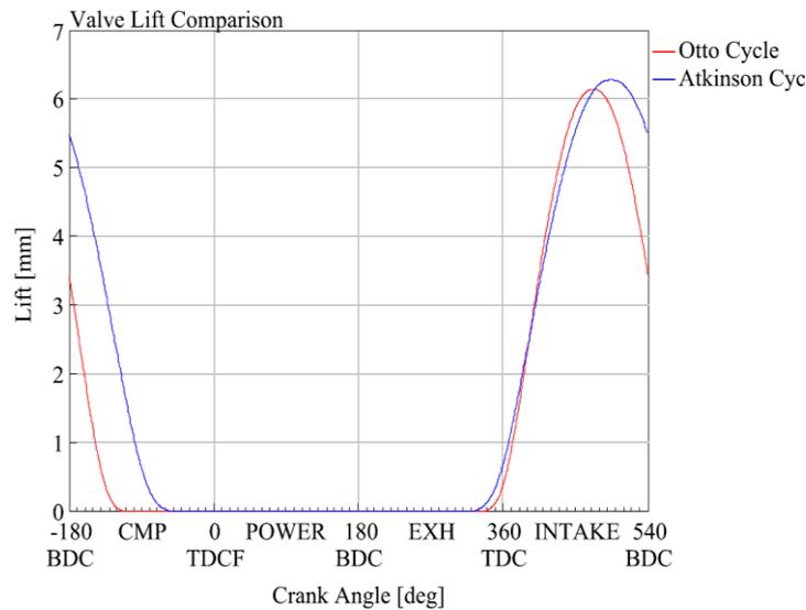
Figure 4.9 Cam Lifts of Otto and Atkinson cycle.
