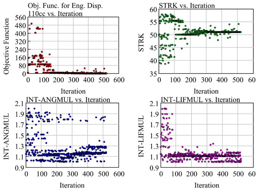
**Figure 4.7** Optimization of LIVC timing via genetic algorithm.
