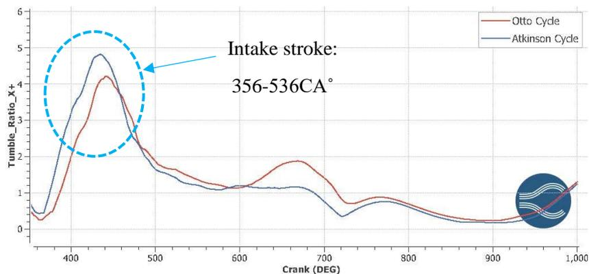
Figure 4.10 Tumble ratio comparison between Otto cycle and Atkinson cycle.
