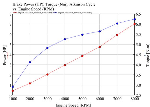
**Figure 4.13** Atkinson power and torque data via GT-Post.
