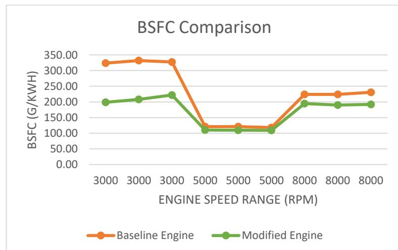
**Figure 4.16** BSFC comparison for baseline and modified engine.
