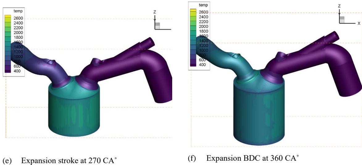
**Figure 4.4** Post-processing using Tecplot, with temperature contours.
