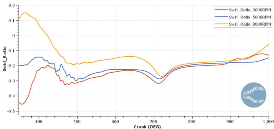
**Figure 4.2** Swirl ratio of baseline engine at 3000, 5000, and 8000 rpm.
