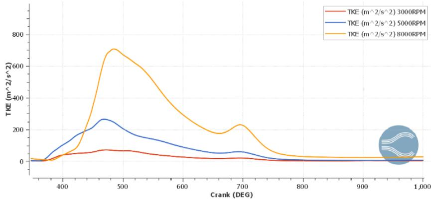
**Figure 4.3** Turbulence kinetic energy of baseline engine at 3000, 5000, and 8000 rpm.
