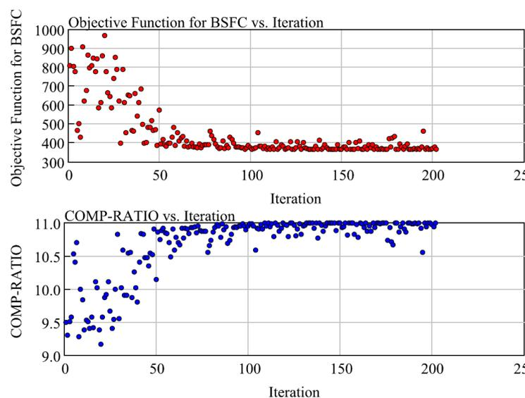
**Figure 4.8** Optimization of compression ratio via genetic algorithm.
