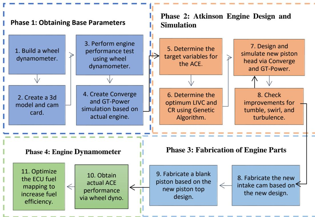
Figure 3.0 Conceptual framework for the design, simulation, and testing of the engine.
