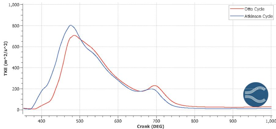
**Figure 4.12** Turbulent kinetic energy comparison between Otto cycle and Atkinson cycle.
