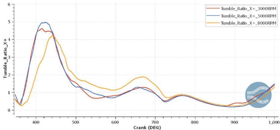
**Figure 4.1** Tumble ratio of baseline engine at 3000, 5000, and 8000 rpm.
