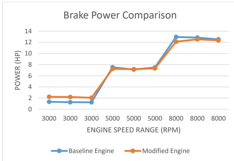
**Figure 4.14** Brake power comparison for baseline and modified engine.
