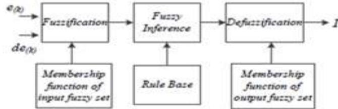
Figure 9. Structure of Fuzzy logic controller
