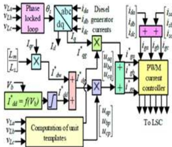
Figure 3. LSC control algorithm
