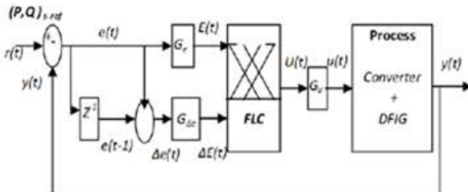
Figure 7. DFIG based microgrid with FLC controller
