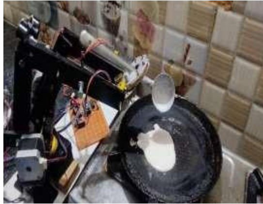
Fig.4.d: Rotating the arm to make the batter into circle
