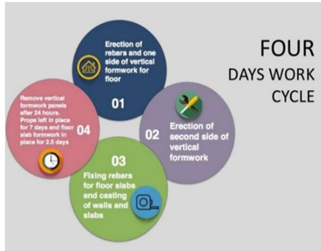
Figure 7. MIVAN Formwork Work Cycle
