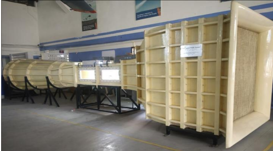
Fig 2 Suction types Low-Speed wind Tunnel
