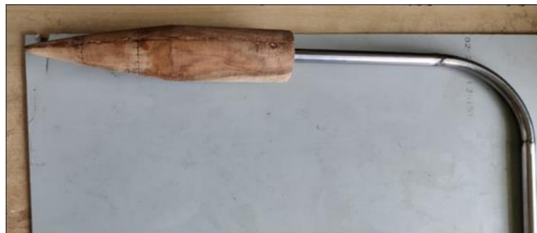
Fig. 3 Fabrication of Sharp Conical Nose Model
