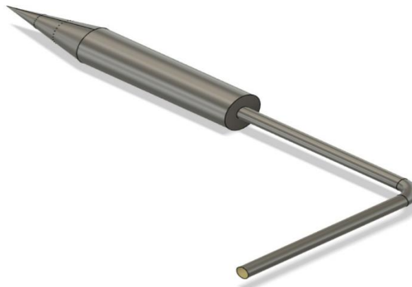
Fig.1 Experimental Model of Sharp Conical Nose
