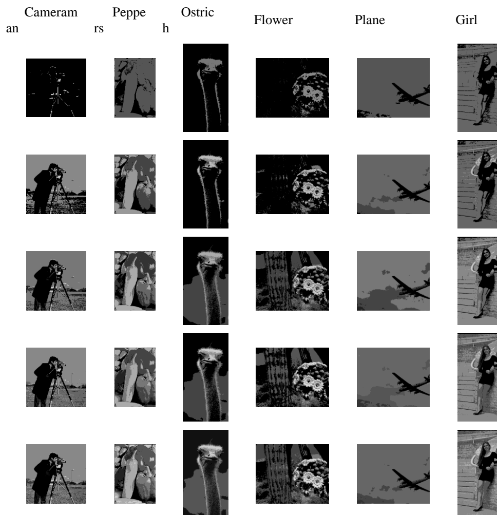
Fig.2. Segmented images with thresholds levels k = 1, 2, 3, 4, and 5 obtained by the proposed EMA algorithm.
