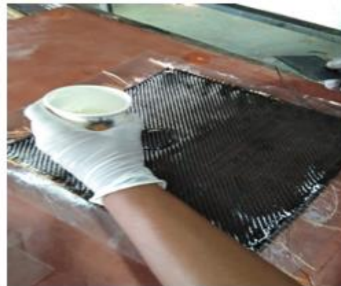
Figure 2.2 Applying resin hardener
