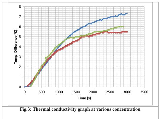
From fig.3 shows that the good thermal behavior at different concentration of cnt. In this fig.red line shows best conductivity at different temperature difference. The high thermal conductivity of the polymer blends can be attributed to comparatively strong hydrogen bonds with cnt. CNT participate in the formation of bonds with-OH groups in the side chains of PVA. In this study, the reduction of hydrogen bonds by the disturbance of cnt was observed in the fig., judging from
