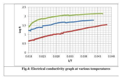
From the Fig.4 shows that electrical conductivity increases due to the addition of CNT in PVA matrix.[8].This is due to the multiwalled CNT coordinated through ionic bonds with hydroxyl
