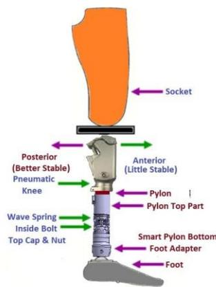
**Figure. 1** A typical transfemoral prosthesis
