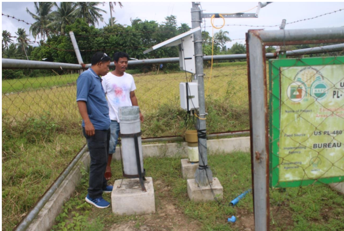
Figure 2. Water Rain Gauge Monitoring device located at Catalotoan, San Jose, Camarines Sur
