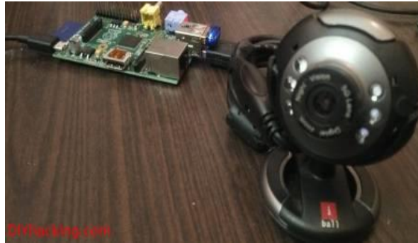
Figure 6: Connecting Camera to raspberry pi.
