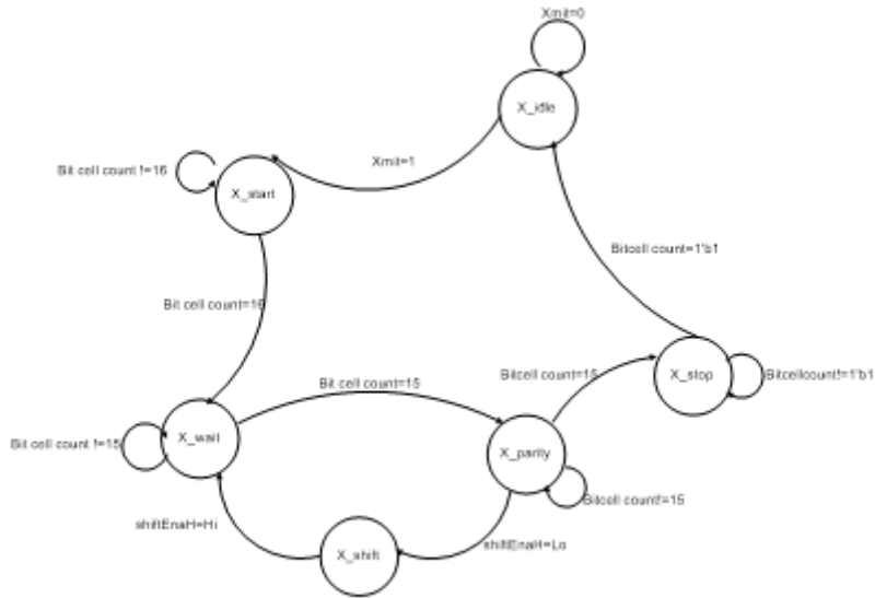
Figure 6. State diagram of UART transmitter
