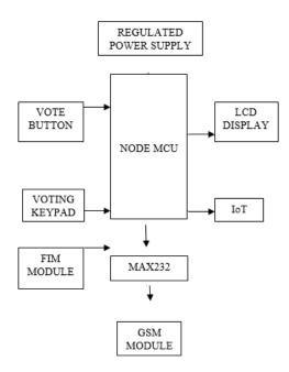
The Regulated Power Supply is used to run the Node MCU. It is a low cost open source IoT platform and also a development board, firmware based in the widely used ESP8266-12E WiFi module. The
