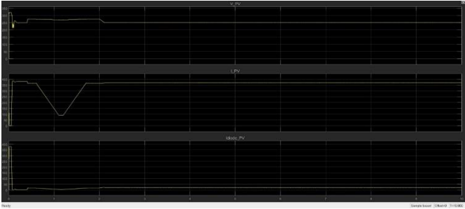
Fig.B.1: Voltage and current from PV array different irradianations
