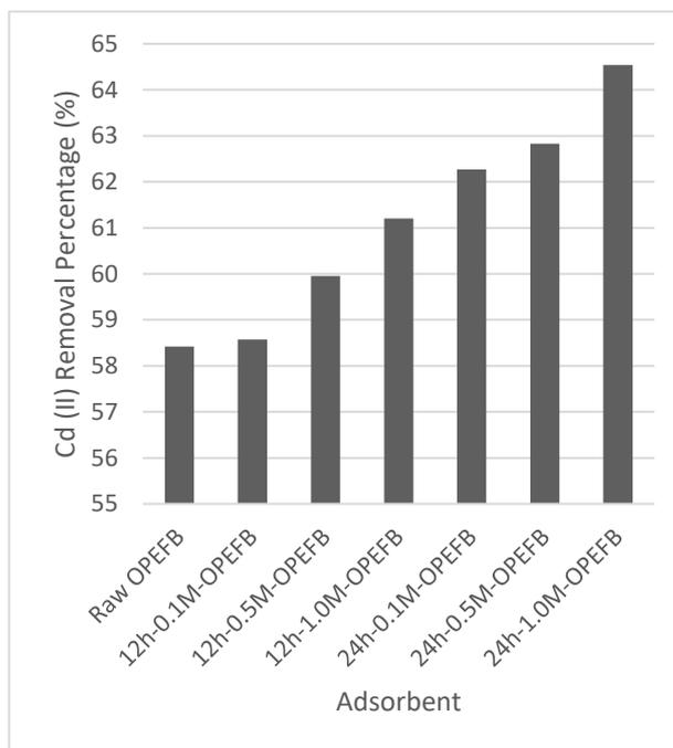
**Fig. 1.** Cd (II) ions removal percentage by different NaOH treatment condition adsorbents (conditions: adsorbent dose = 0.01 g per 100 ml solution, adsorbate concentration = 5 mg·L<sup>-1</sup>, pH = 4, contact time t = 2 h, temperature T = 25 °C, and stirring rate = 150 rpm)
