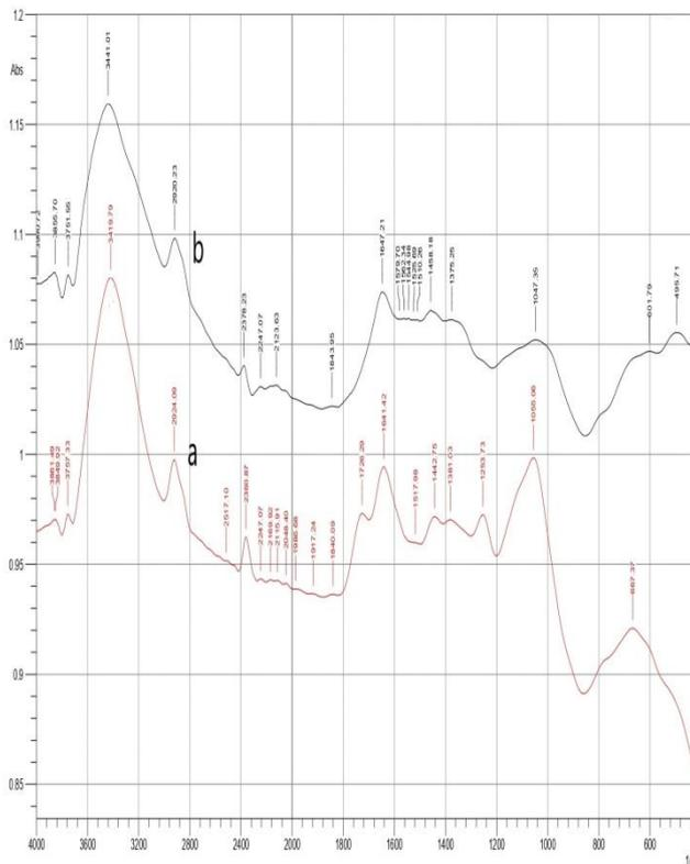
**Fig. 4.** FTIR spectra of raw OPEFB (a) and treated OPEFB (24h-1.0M-OPEFB) (b)
