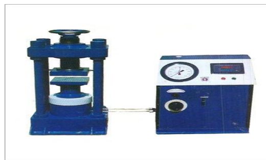
Fig 4.4: Sample testing on CTM for Split tensile Strength
