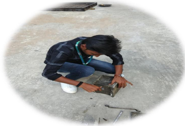
Fig: 3.8. De-moulding of specimens
