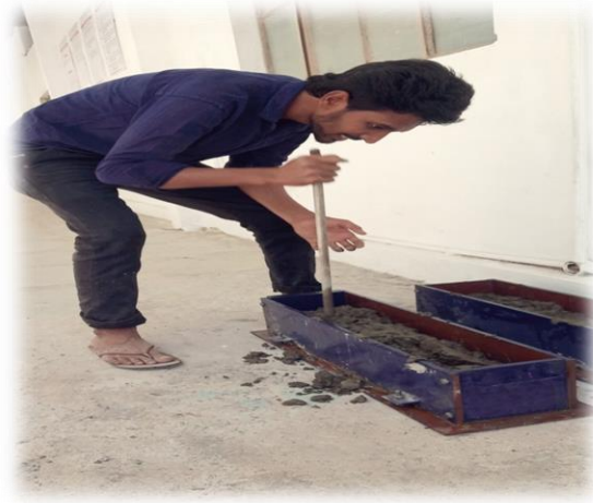
Fig: 3.7. Casting and Compaction of Beams
