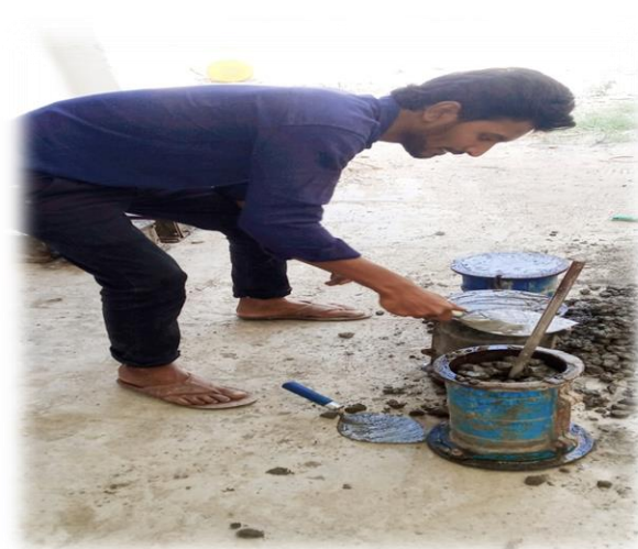
Fig:3.6 Casting and Compaction of Cylinders
