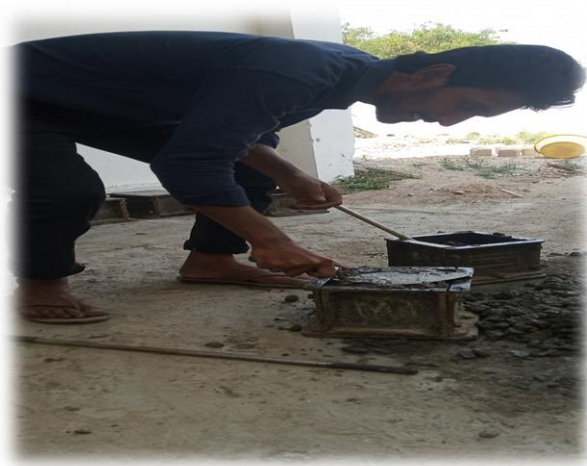
Fig: 3.5.Casting and Compaction of Cubes
