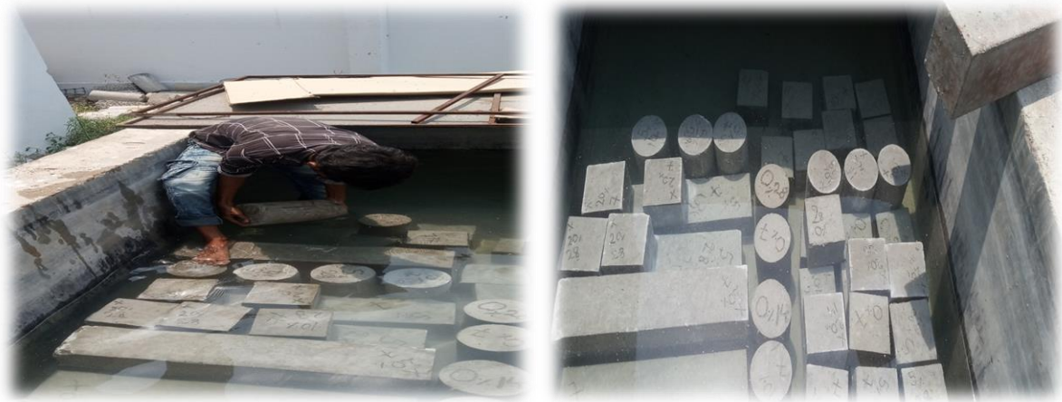
Fig: 3.9 curing tank
