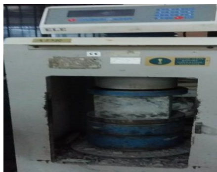
Fig. 2.9. Compressive Strength Test
