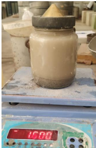
Fig. 2.3.4 Pycnometer with wet Stone Dust and Stone Dust in a try
