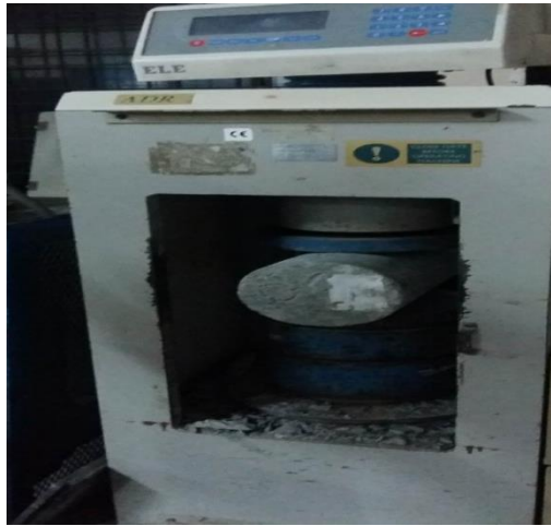
Fig. 2.10. Split tensile strength Test
