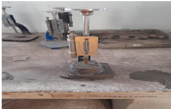
Fig 2.8: initial setting time of cement sample
