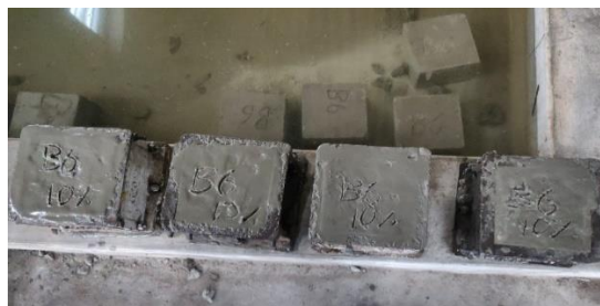
Figure 2.6: Curing of Concrete Cubes
