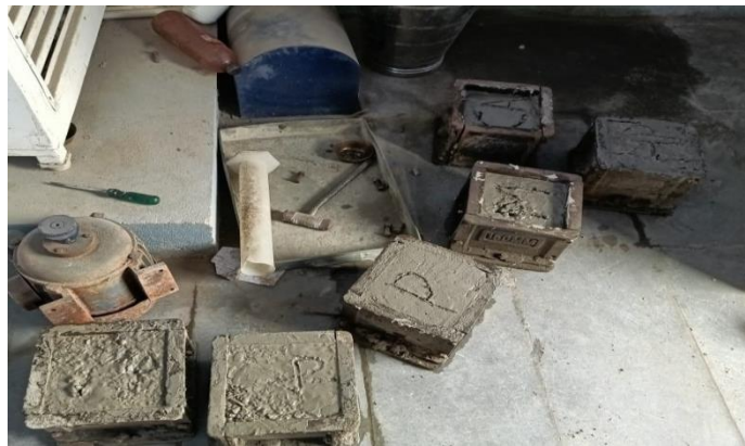
Figure 2.4: Casting of concrete cubes
