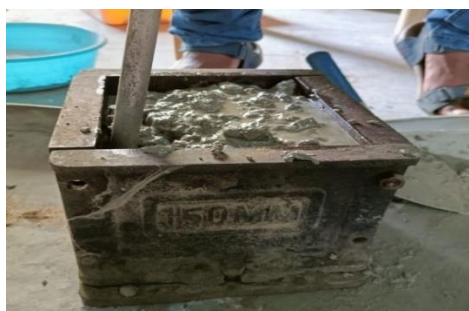
Figure 2.5: Compacting concrete cube
