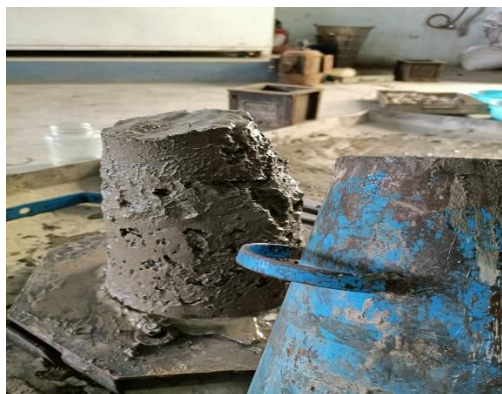
Figure-4.1.: Concrete Slump cone test
